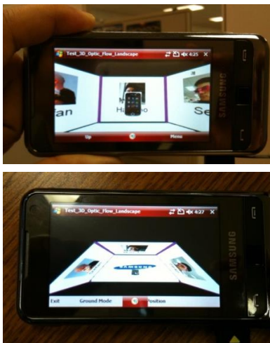
Fig. 8. Gradual transition from first-person view (device held vertically, top) to map view (device held horizontal, bottom), with the virtual camera perspective smoothly rising to an overhead position.
