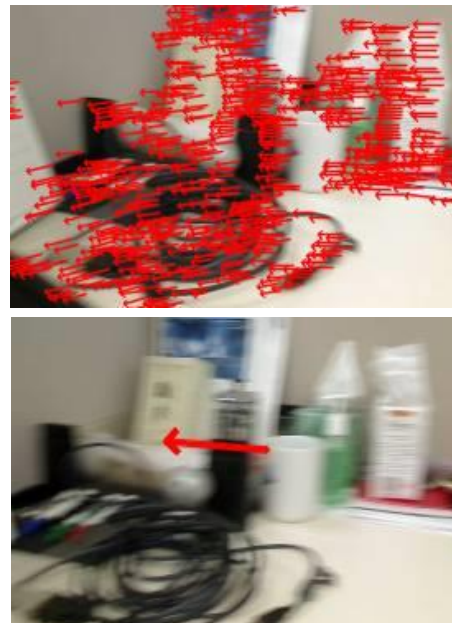
Fig 2. Example of optical flow field (top) and resulting overall optical flow 2D vector (bottom).
