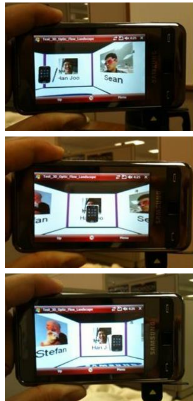
Fig. 7. Example of a sideways shifting motion, at a slow yet constant speed. This is detectable reliably with optical flow from an imager in parallel to the motion plane, but not reliably with inertial sensors alone.
